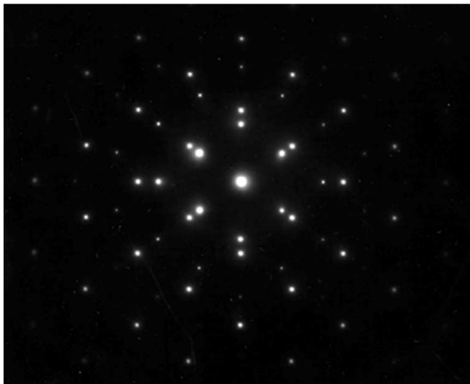
Fig. 7. Selected area electron diffraction pattern of the 3C-SiC/Si interface.
