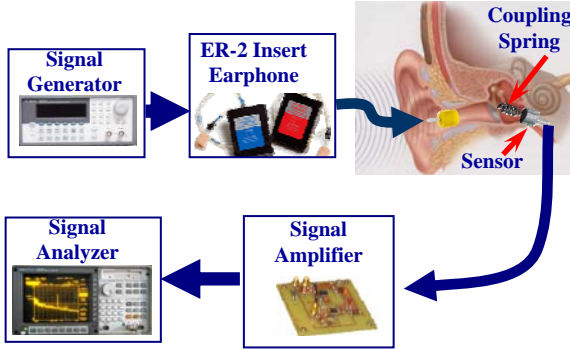
Fig.7. Measurement set-ups for temporal bone experiment
